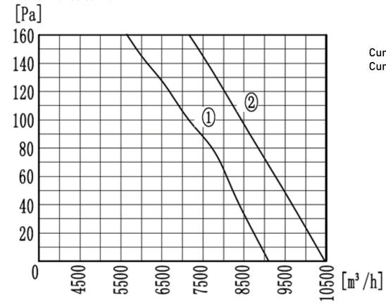
Curve 1: 50HZ Curve 2: 60HZ
